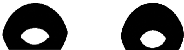
Fig. 2 Reversible switching of contact angle of photoresponsive compound 1a for water before irradiation (left) and after 366 nm light irradiation (right).
